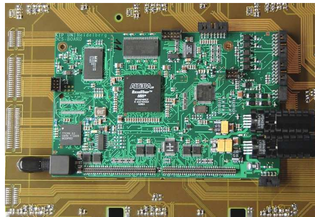
DCS control board (~750 used in ALICE)
